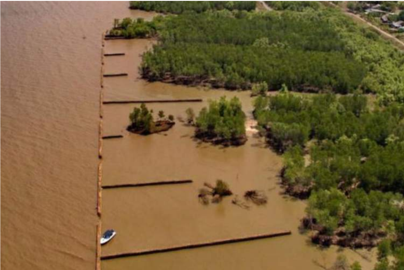
Wave dampening effect of bamboo T-fences, Ca Mau Province, Viet Nam. Photo by R. Sorgenfrei. Source: Schmitt, K. and Albers, T. 2023. Mangroves and ecosystem-based coastal protection in the Mekong River Delta, Vietnam. In O. B. B. Yllano (Ed.), Mangrove Biology, Ecosystem, and Conservation. IntechOpen. https://doi.org/10.5772/intechopen.110820
